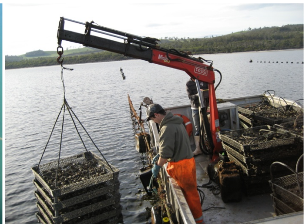
As the oysters are in deep water we use a boat (barge) equipped with a crane to access the oysters.
